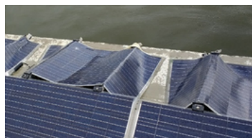
e) Damage on PV modules due to wave slamming
