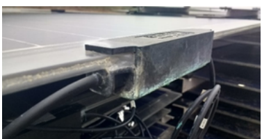
g) Corroded junction box
