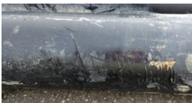
a) Rubbing damage on an HDPE part
