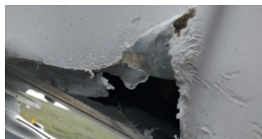
b) Rubbing and stress damage on an HDPE part
