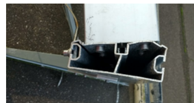
c) Torsion damage on an aluminium part
