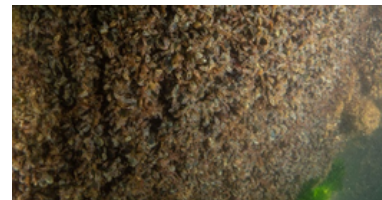
f) Biofouling of underwater component
