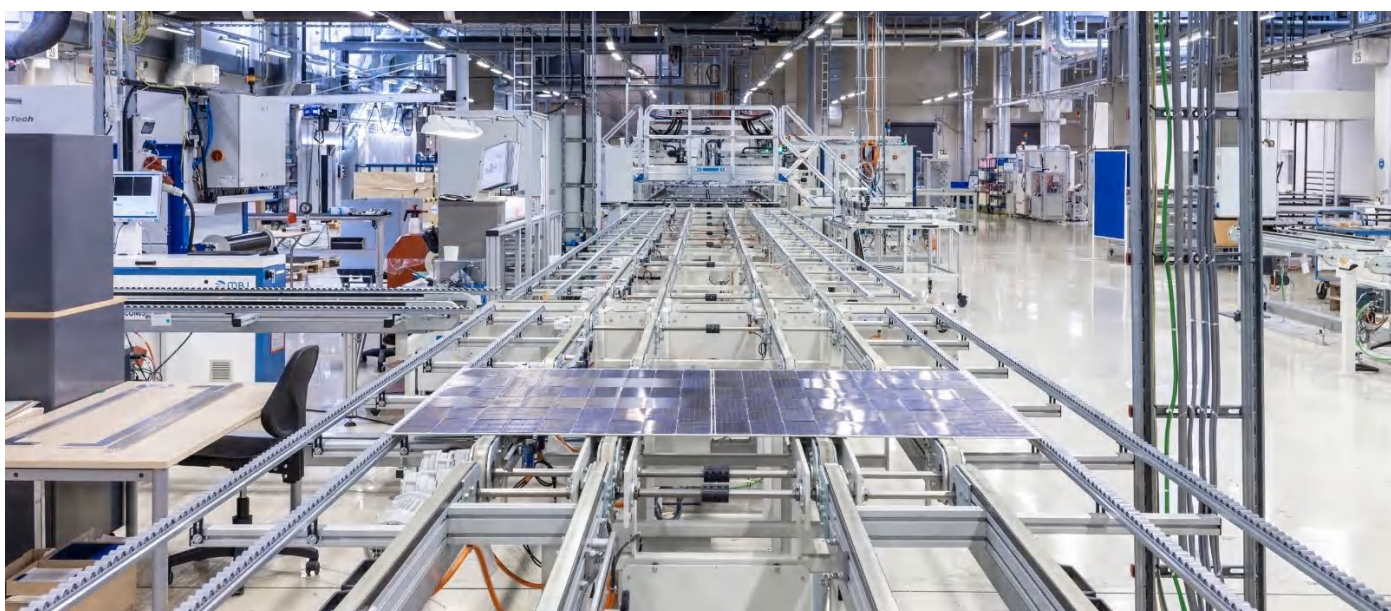
Figure 13: Qcells pilot line in Thalheim, Germany, from project PEPPERONI, which Horizon Europe supported with 13 million EUR to deliver a pilot line for the production of perovskite-silicon tandem cells and modules on industrial scale.
