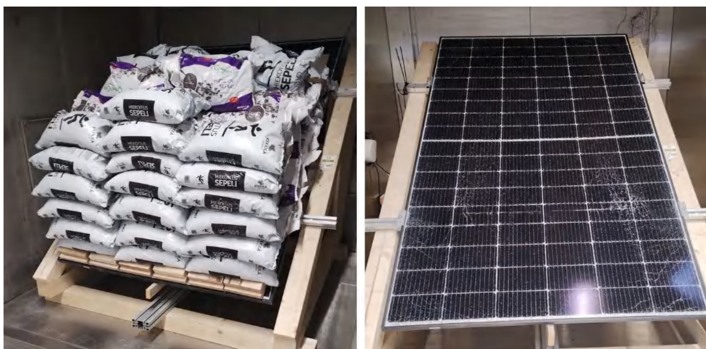
Figure 15: Snow load testing of thin glass PV modules. Photo: Shuo Wang, Turku University of Applied Sciences.
